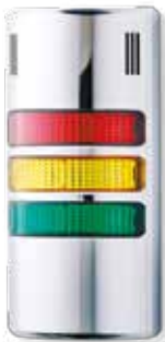
Order number: HD90-Q47 Colours: red/yellow/green Function: LED steady beacon, buzzer steady or pulsing tone Housing colour: chrome Nominal voltage: 24 V AC/DC
