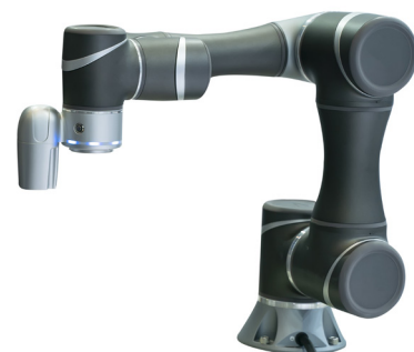
Figure 4: Articulated arm robots often have up to six serial axes and enable complex motion sequences.
