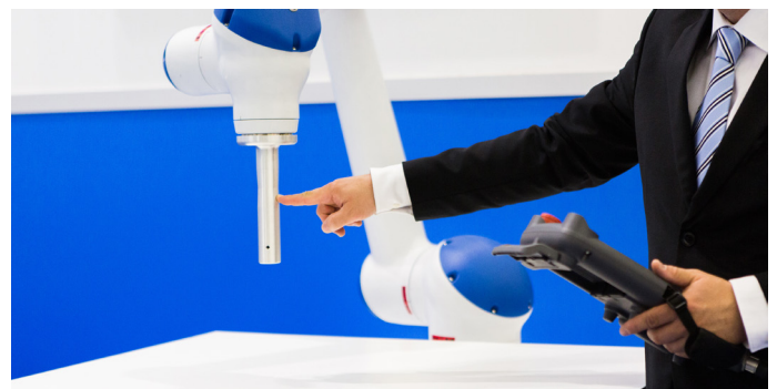
Figure 6: Teaching a robot with the aid of an operating terminal takes a relatively long time, which is why offline methods are increasingly being used.
