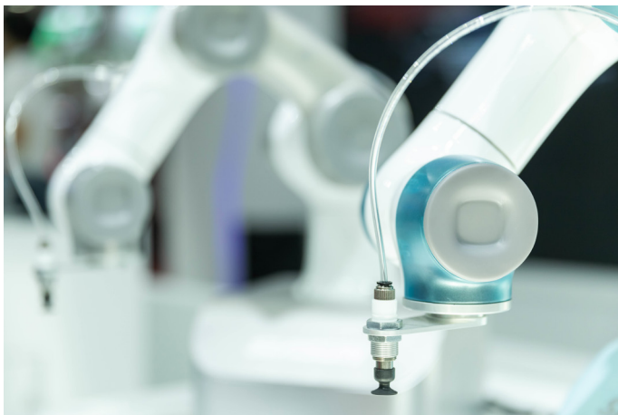
Figure 5: The use of vacuum grippers to pick up objects is widespread among robots.
