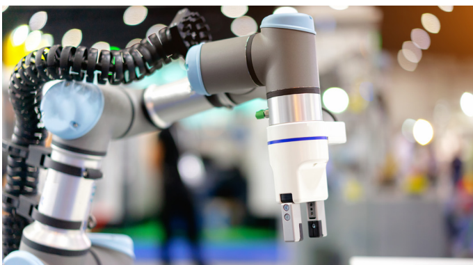
Figure 8: The constant movements of a robot require special torsion- and bending-resistant cables and, if necessary, drag chains.
