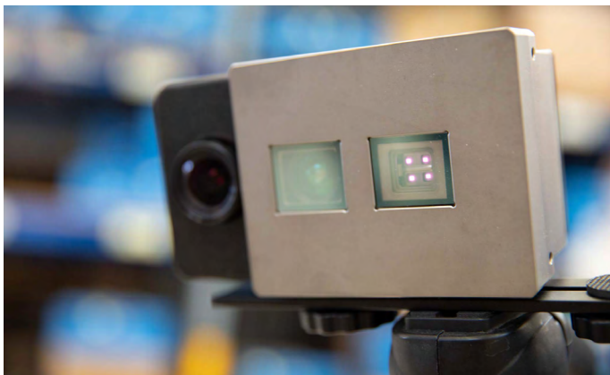
Fig. 2: Basler blaze: The perfect 3D camera for applications in logistics, here in combination with a Basler ace color camera.
