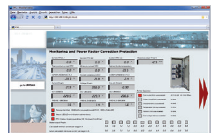
Fig.: Monitoring of limit values via UMG 604 homepage
