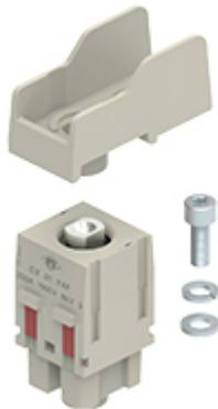
Female modular insert, Mixo series, screw terminal connections - 90° angled for cable lug, 1 pole, 2 modules, 200 A 1000 V 8 kV 3
