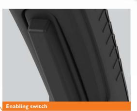
The three-stage enabling switch ensures optimum safety during the operation of machines and devices in hazardous areas. Only an actively operated middle position gives approval to a higher-level safe control.
