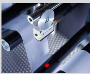
**FT 25-R(L)A for dancer roll regulation** The precise control of the FT 25-R(L)A ensures a constant tension of the paper roll during unwinding.
