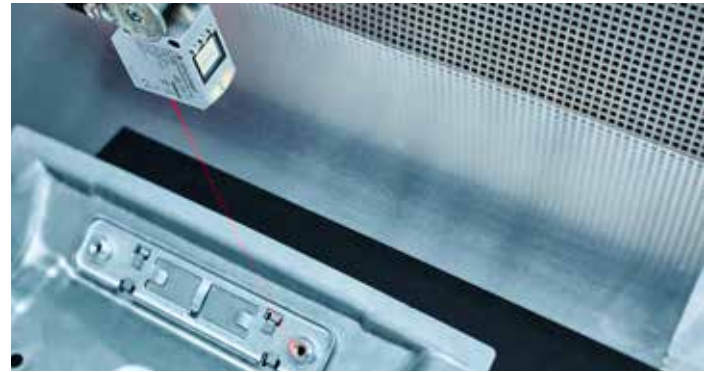
Detecting the presence of weld nuts
