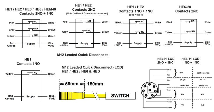
**CONTACT OPERATION -** The N/O contact(s) on Mechan safety switches are open when the actuator is away from the switch. When the actuator is within the specified operation distance, the N/O contact(s) will close and N/C contact will open.
