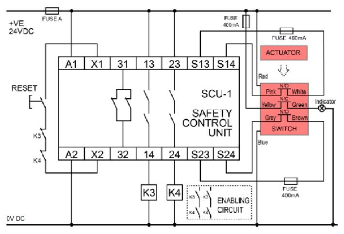
Fuse A: Main fuse for overall circuit including the contactors. 400mA Fuses: Fast acting (quick Blow) to protect all switch contacts.
