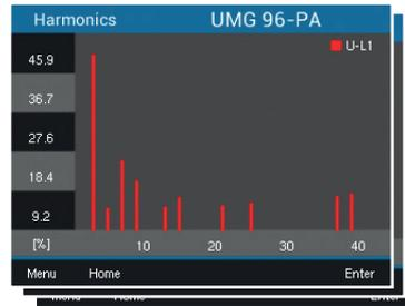
Display of the harmonics up to the 40th harmonic (voltage L1, L2, L3)
