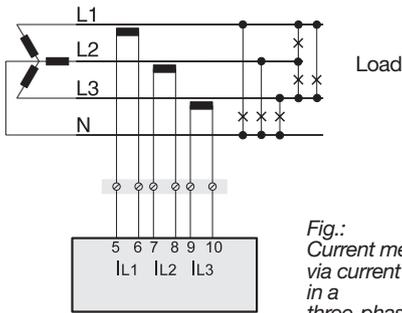
*Fig.: Current measurement via current transformer in a three-phase 4-conductor system*
