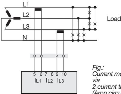
*Fig.: Current measurement via 2 current transformers (Aron circuit) in a three-phase 4-conductor system*
