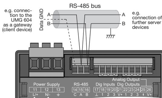
Fig. RS-485 interface, 3-pole plug contact
