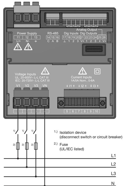
Fig. Connection example for voltage measurement.
