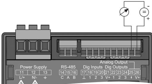
Fig. Analog output connection
