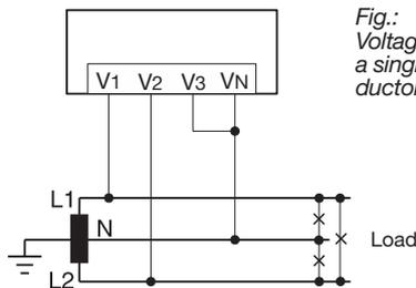
Fig.: Voltage measurement in a single-phase 3-conductor system
