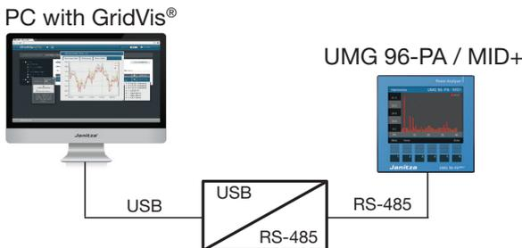
2. Use of the UMG 96-PA/-MID+ (server device) via a UMG with gateway functionality (e.g. UMG 512 client device):
