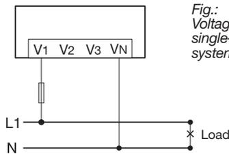
Fig.: Voltage measurement in a single-phase 2-conductor system
