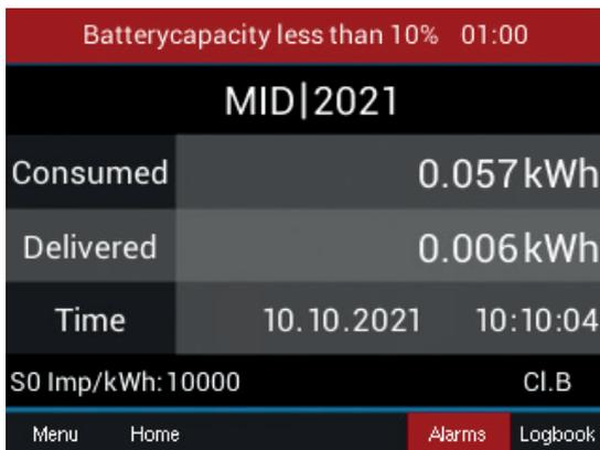
Fig. Warning message "Battery capacity less than 10%"
