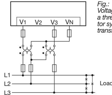
Fig.: Voltage measurement in a three-phase 3-conductor system with voltage transformer.
