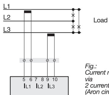
*Fig.: Current measurement via 2 current transformers (Aron circuit) in a three-phase 3-conductor system*
