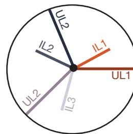
Current and voltage are shifted against each other. The current is ahead the voltage, i.e. the network is capacitively loaded.
