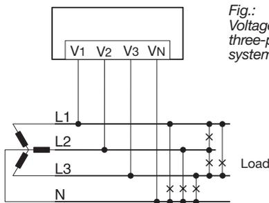
Fig.: Voltage measurement in three-phase 4-conductor system
