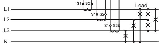
Fig. Connection example, "Current measurement via current transformer".
