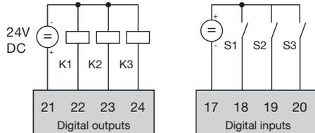
Fig. Digital outputs and inputs
