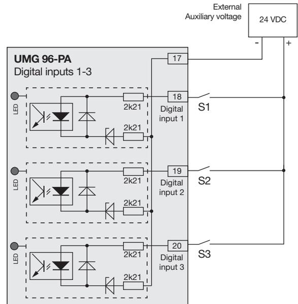
Fig. Example for the connection of the external switching contacts S1-S3 to the digital inputs 1, 2 and 3.
