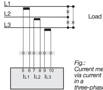
*Fig.: Current measurement via current transformer in a three-phase 3-conductor system*
