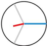
Voltage and current have a deviation of about 180° in the phase position.
