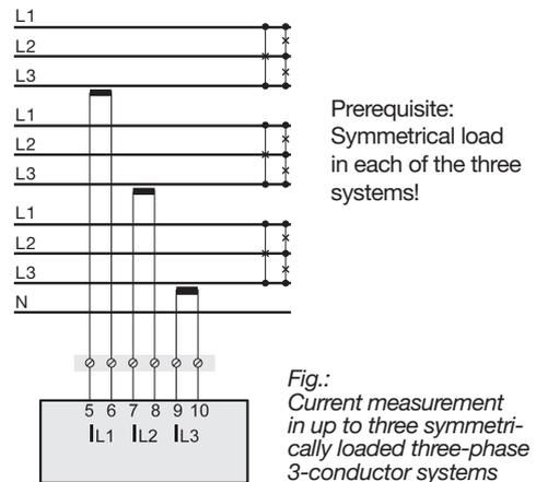
*Fig.: Current measurement in up to three symmetrically loaded three-phase 3-conductor systems (only UMG 96-PA, not UMG 96-PA-MID+)*
