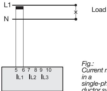
*Fig.: Current measurement in a single-phase 2-conductor system*
