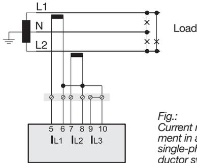
*Fig.: Current measurement in a single-phase 3-conductor system*
