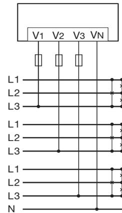
Fig.: Voltage measurement in up to three symmetrically loaded three-phase 3-conductor systems (only UMG 96-PA, not UMG 96-PA-MID+)
