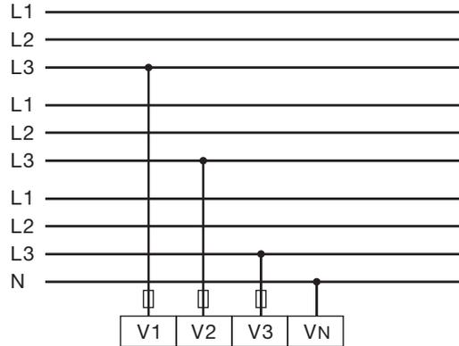
Fig. Three systems with uniform loading of the phases. The unapplied measured values L2/L3 or L1/L3 or L1/L2 of the respective systems are calculated.
