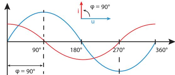
With a combination of the states, the phase angle “current to voltage” can assume values between -90° and +90°.
