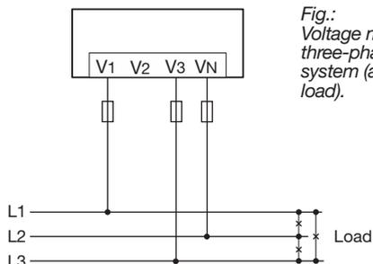
Fig.: Voltage measurement in a three-phase 3-conductor system (asymmetrical load).
