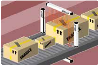
Measurement of the height of objects in transit on conveyor systems. Two-dimensional detection of objects in transit with use of 2 sets of light curtains
