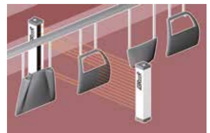
Detection of position and profile of workpieces in automated painting systems
