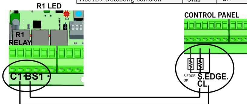
The equipment can be connected to the control panel with input for safety edge 8k2 or directly into a safety input normally closed contact as if it were a photocell or stop signal.
