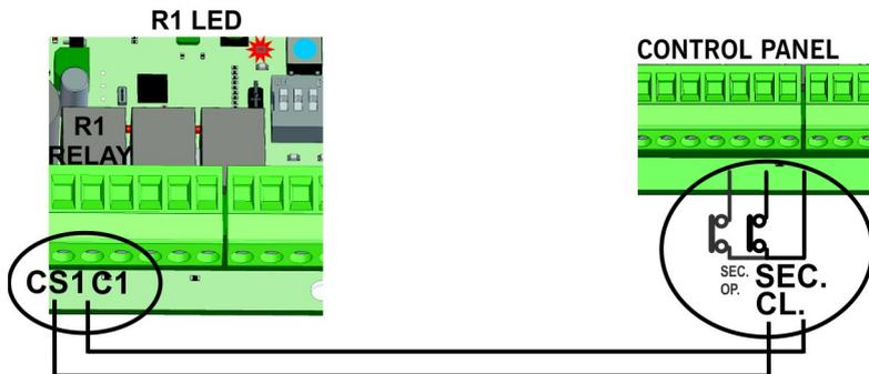
Example: connection to control panel with input for safety edge 8k2
