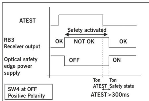
Allowed in ON mode because they are permanently active. The radio communication is tested every 7 seconds.
