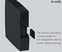
The memory card allows an easy transfer of
