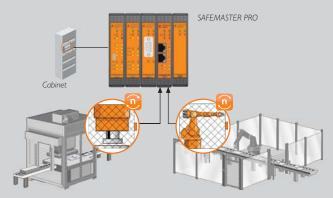
Safe speed monitoring with the new SAFEMASTER PRO expansion modules. Monitoring of 2 axes by means of encoders (alternatively with proximity sensors). Simple configuration with the free
