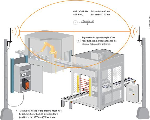
Is the optimal height differential of the antennas, two antennas should be installed within this height deferential if possible. This is only advisory and may have to be altered with regards to ground clutter noise and reflections.
