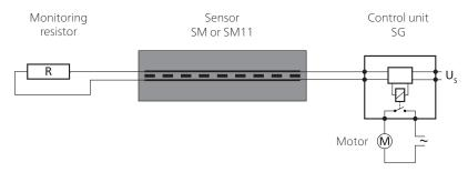
The monitoring resistor must be compatible with the control unit. The standard type is 8k2.
