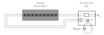
The 4-wire technology can only be used together with control unit SG-EFS 104/4L.
