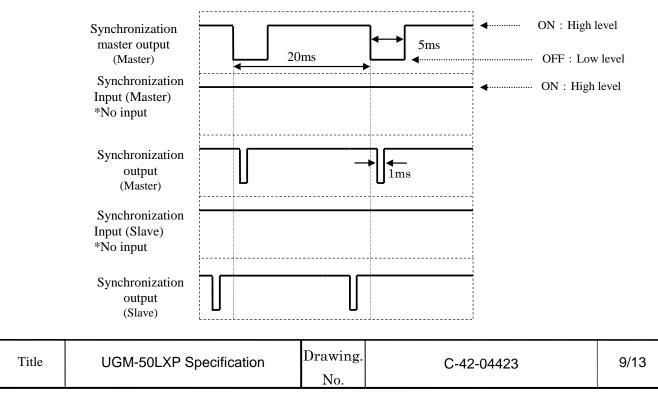
When the synchronization master output of the master is connected to the synchronization input of the slave, the master sensor can synchronize falling edges of the synchronization master output signal with falling edges of the synchronization output signal.
