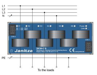
Fig.: Operating current measurement, e.g., 6 x 1-phase
