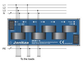
Fig.: Residual current measurement
