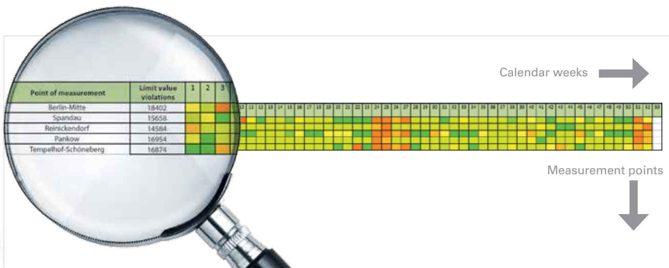
Fig.: Heatmap, i.e. colour (traffic light principle) illustration of how good or bad the power quality was at a particular measurement point in a calendar week. This principle guarantees a quick overview of the complete supply area.
