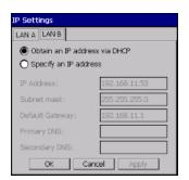
If the operator panel is equipped with two Ethernet ports, then a second tab is shown in the IP settings dialog. The default setting for LAN B is "Obtain and IP address via DCHP".
