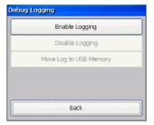
The Debug Logging dialog enables the function to enable and disable the debug logging on the operator panel. It also enables the function to move a previously created set of debug log files from the operator panel to an USB flash drive.
