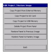
The edit project / restore image dialog allows modifying the project in an operator panel and, if needed, restore the panel image to a previous version.
