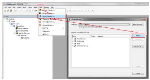
The installation button in CODESYS 3.5 SP10 Patch 1
