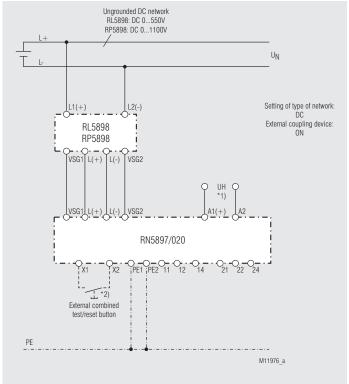
\*1) Auxiliary voltage  $U_{_{H}}$  (A1(+)/A2) ) can also be sourced from the monitored voltage system. The voltage range of the auxiliary supply has to be taken into account.
